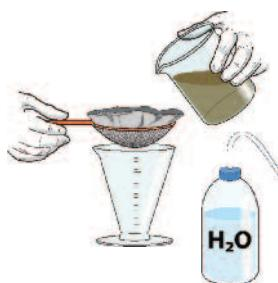
Filter the faecal suspension using a wire mesh (aperture of 250 µm) and add tap water up to 250 ml
