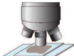
Discard the supernatant and transfer 10-15 ml of sediment in a Petri plate or add some drops of sediment on a glass slide, add a coverslip and examine under the microscope.
