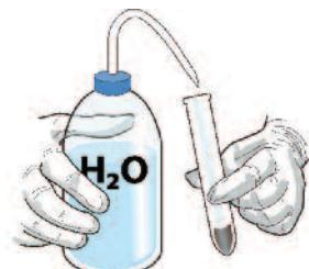
Refill the tube with tap water up to 9-10 ml and allow to settle for 2 minutes
