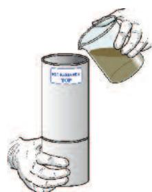
Tap the Flukefinder against the side of the sink to expedite the passing of water through the screens and hold the column under the cold running tap until about half full (repeat this step for 4-5 times)
