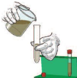
Swirl suspension and pour into a tube and allow to settle for 3-4 minutes
