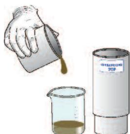
Invert the bottom unit over a cup and backwash the eggs and debris from the screen into the cup
